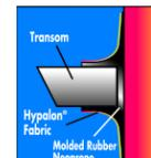
We have always secured our transoms with a unique Neoprene rubber mold and transom tape combination; not just one or the other. This makes them ideal for handling the extra weight associated with 4-stroke motors.
